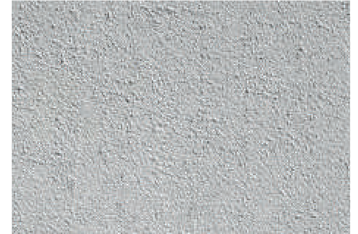
Self-coloured, insulated acrylic render
